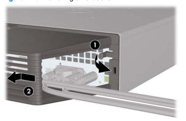
Figure 7-28 Removing a Port Cover
